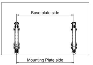
Ensure that the two LIN-X bodies are parallel by measuring both the base and mounting plate distances.
