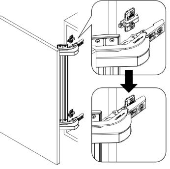
Ensure that the LIN-X body is securely attached to the mounting plates.
