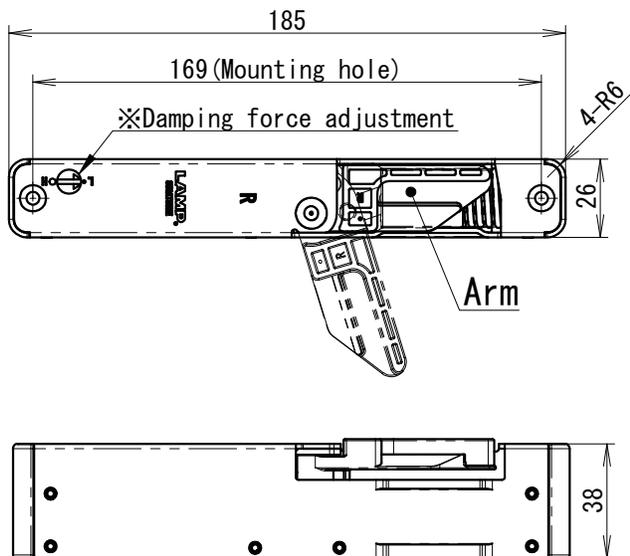
※CAUTION : Set the adjustment screw to either H or L position, not any intermediate position.
