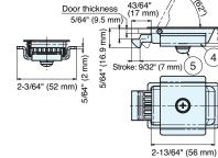
Insert the latch through the cutout, and fix it with the back plate and screw.
