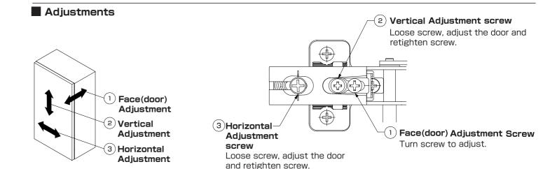
Ensure that all the screws are securely tightened. Remove all the protection tape after assembly is finished.
