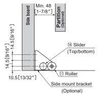
Note: Slider should always be installed towards front of the cabinet.
