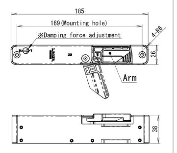
\*CAUTION: Set the adjustment screw to either H or L position, not any intermediate position.
