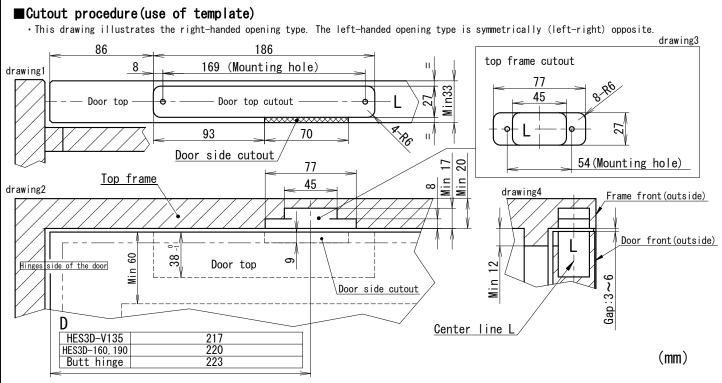
· Separate the door template from the frame template, affix it to the top of the door and cut door accordingly. The damper body should be
