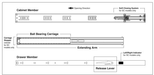
2. Position cabinet member assemblies as shown. Using the horizontal slots, the closed position of the drawer can be adjusted to achieve proper 1/8" (3mm) reveal and engage the hold-in detent.
