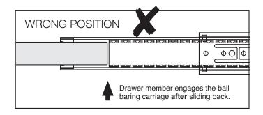
4. Ensure that both right and left sides are aligned as parallel as possible for best movement.
