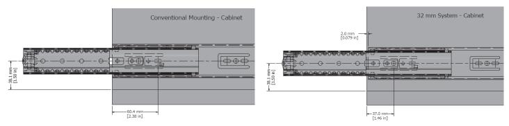
3. Ensure ball bearing carriage is pushed all the way to the front and lodged against the carriage stopper when re-installing the drawer member into the cabinet member, as shown above.
