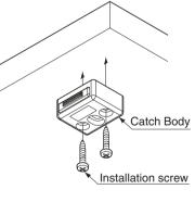
Use both side holes to secure the body catch. Size 4 screws (not included) are necessary
