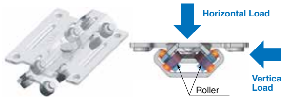
Rollers are located at two different angles to resist both horizontal and vertical loads.
