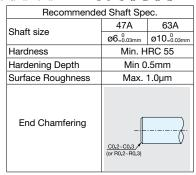
When inserting shaft, insert by rotating shaft in the opposite direction of the dampening direction. Shaft must be supported by stationary part. Damper can only take torque load.
