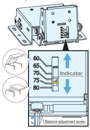
Angle of peak torque is adjustable with hex key 5 mm (13/64"). This feature allows for position adjustment to change the center of gravity.
