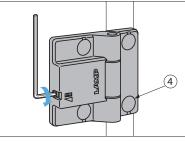
Closing speed of doors is adjustable with a hex key (size: 2.5).
